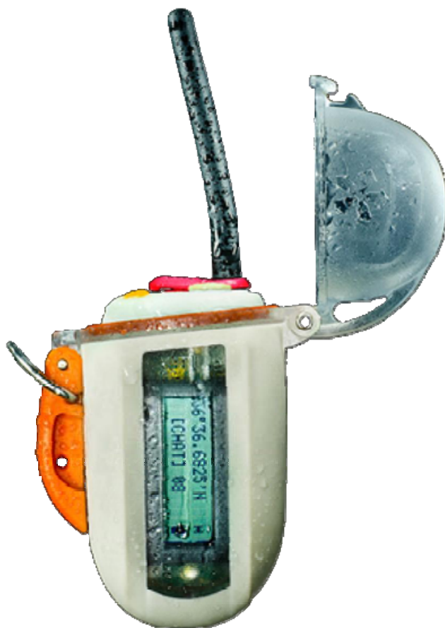
Nautilus Lifeline two-way VHF marine radio and GPS locator.
